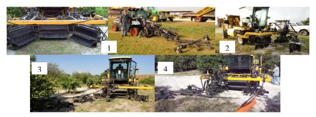
Fig. 2. The modified Oxbo 3200: 1. flap-wheel. 2. centipede. 3. combination centipede and wheel-sweep. 4. wheel-sweep.
